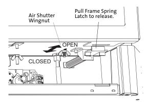
Figure 11. Frame latch and air shutter stem location.
